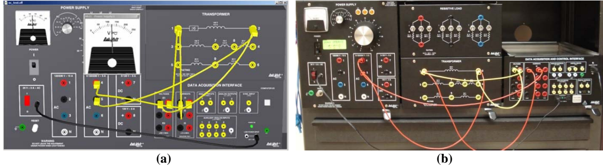
Figure 2- Open circuit test setup in (a) Simulation software (b) Actual hardware
