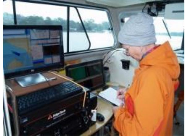
The actual process of surveying the sound involved long hours of slowly driving the boat back and forth on long parallel tracks. On each leg, the sonar produced a long, narrow strip indicating the depth and character of the sound bottom. Using high-resolution Global Positioning System data that pinpointed the boat's exact location, the system assembled the digital strips of data into a complete picture of the survey area.
