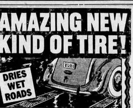
How Amazing New Life-Saver Tread Gives You a Dry Track **On Wet Roads.** It's actually a "road dryer"! Its never-ending spiral bars act like a battery of windshield wipers, sweep the water right and left, force it out through the deep grooves, making a dry track for the rubber to grip. That's why this new Goodrich Safety Silvertown will stop you seconds quicker on wet roads than you've ever stopped before!
