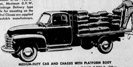
MEDIUM-DUTY CAB AND CHASSIS WITH PLATFORM BODY Model 3508—137-inch wheelbase, Maximum G.V.W. 8,800 lb. Other models available up to 161-inch wheelbase and 16,000 lb. G.V.W.
