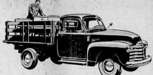
MEDIUM-DUTY DE LUXE STAKE Model 3609—125 1/2-inch wheelbase, Maximum G.V.W. 5,800 lb. Other models available up to 161-inch wheelbase and 16,000 lb. G.V.W.
