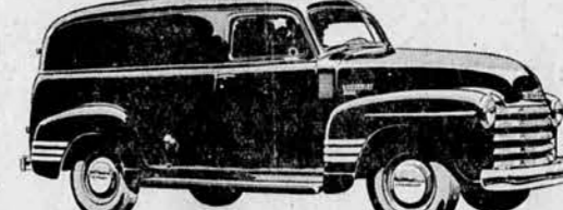
LIGHT-DUTY DE LUXE PANEL Model 3105—116-inch wheelbase, Maximum G.V.W. 4,600 lb. Also available in Medium-Duty model 3805—137-inch wheelbase, Maximum G.V.W. 6,700 lb.
