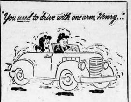
BUT HENRY HAS BOTH HANDS BUSY NOW . . . trying to keep the old bus on the road because his wheels are out-of-line. Misaligned wheels cause "road weave," forcing the driver to "fight" the steering wheel. Out-of-line wheels eat up rubber, too, because the tires are literally dragged sidewise down the road. It isn't only annoying it's expensive.
