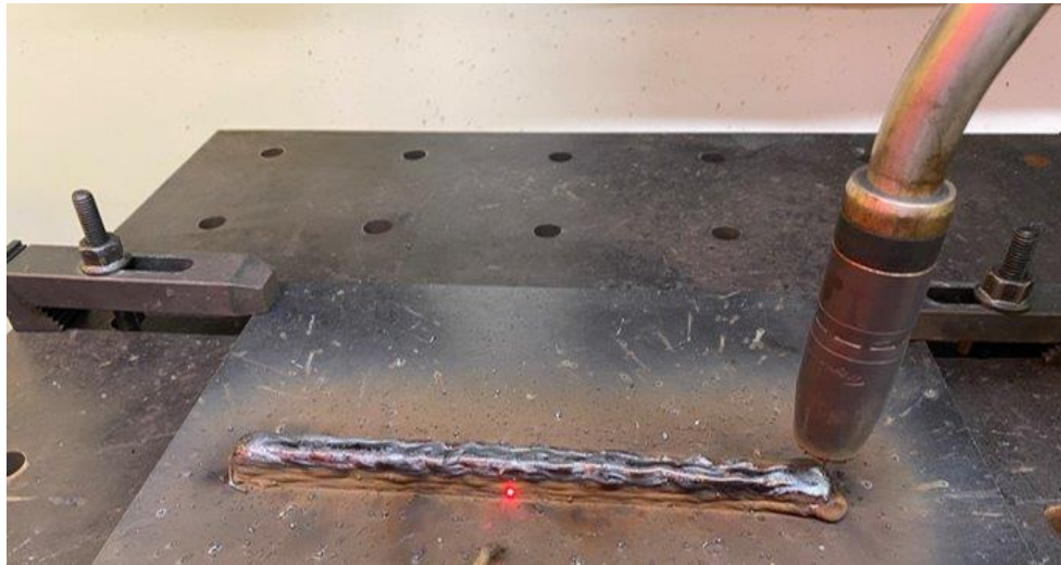
Figure 7. As-Built WAAM Sample
