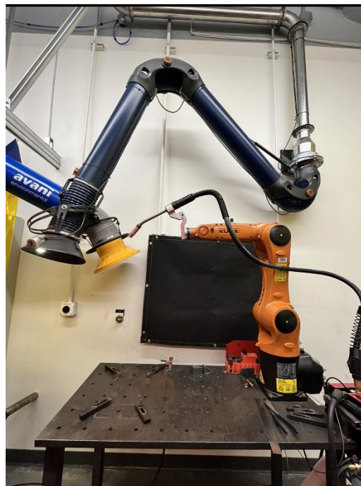
Figure 6. WAAM system used for fabrication of samples
