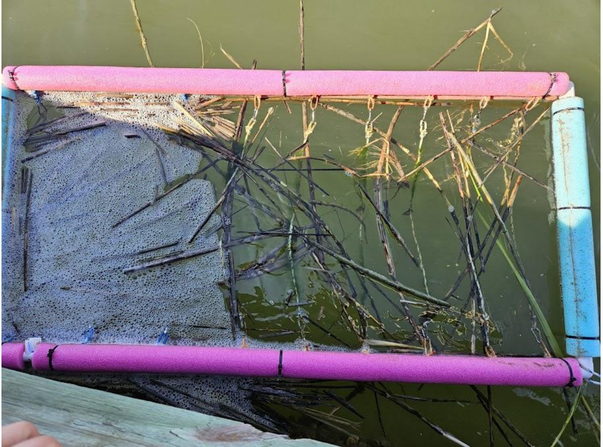
Figure 2.23 Accumulation of decaying vegetation, seafoam, and other debris within the seaweed array at Priest's Landing. This debris had to be removed on a regular basis and may have both hampered growth of the Ulva and affected pH measurements taken inside the array.
