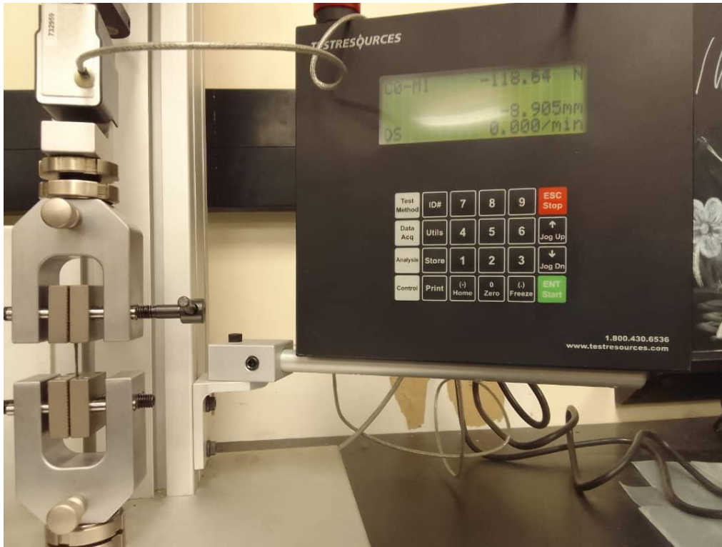
Figure 22. A tensile analyzer from Test Resources ®
