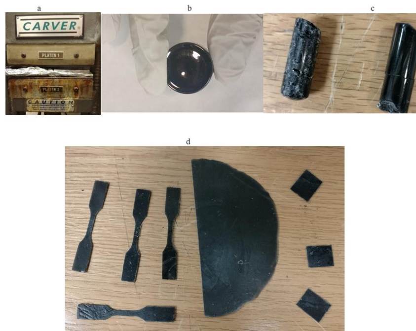
Figure 18. Specimen preparation. a. Molding of composites b. A conventional oven composite taken from vial c. A microwave oven composite d. Preparation of specimen for characterization.
