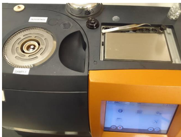
Figure 20. TA Instruments ® DSC 250 Differential Scanning Calorimeter.
