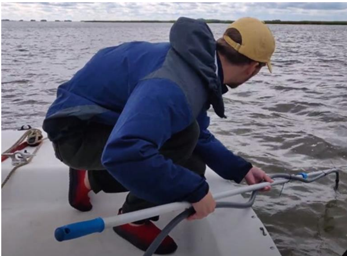
Figure 2.3: Collecting a close-range hyperspectral reflectance scan with Ocean Optics USB2000 fiber optics, just below the water's surface.
