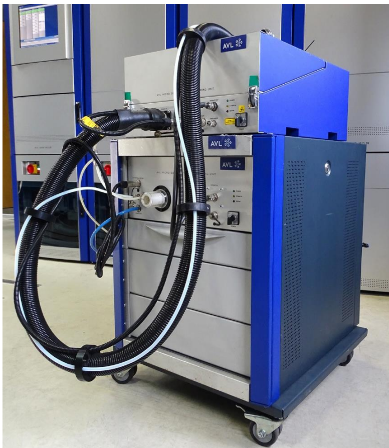
Figure 39: AVL Micro Soot Sensor 483 (BOSMAL 2018)
