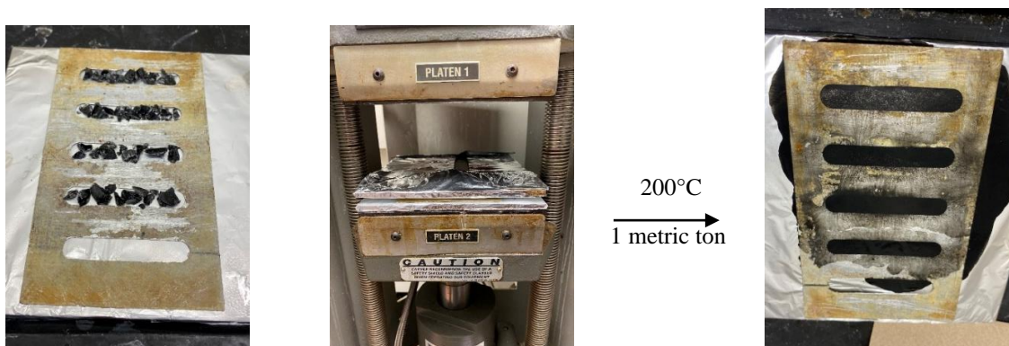
Figure 16. Composite preparation for characterization from 5g composites.
