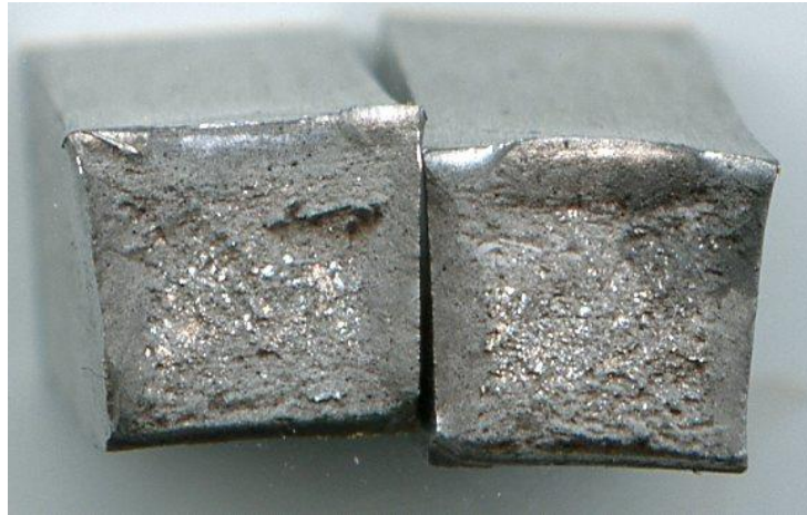
Figure 56: Charpy impact sample 6, 100°C
