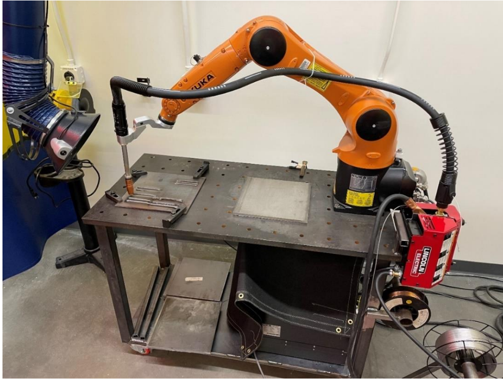
Figure 9: Welding cell used as experimental WAAM setup
