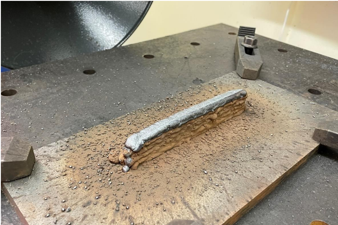
Figure 28: Double Bead wall test, 375WP, excess heat buildup, end geometry failure
