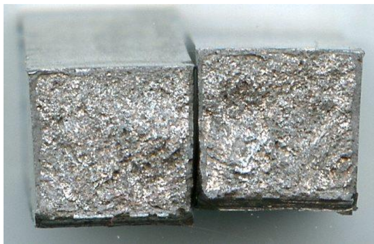
Figure 54: Charpy impact sample 1, 22°C
