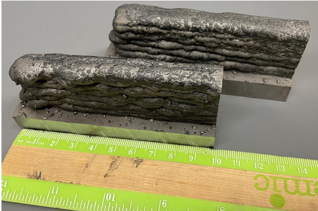
Figure 29: Double Bead wall test, 375WP cleaned and cut to be used for impact testing
