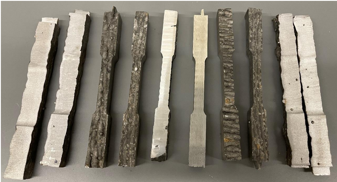
Figure 31: 56 layer double bead wall, waterjet into wishbone tensile coupons
