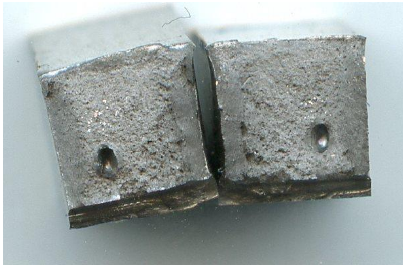
Figure 57: Charpy impact sample 8, 200°C
