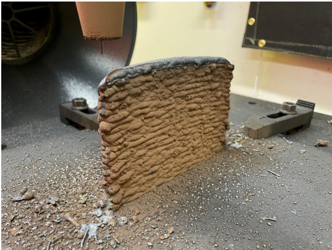
Figure 30: double bead deposition wall, 300WP, 115mm peak height, 56-layer
