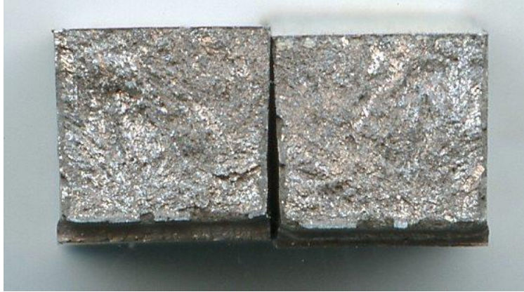
Figure 55: Charpy impact sample 3, 0°C
