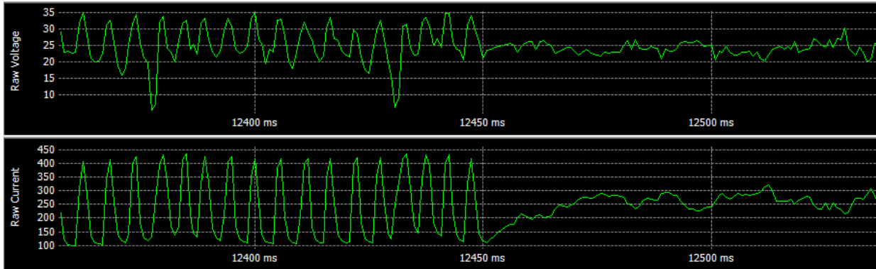
Figure 13: Lincoln Weldview trace graph. With a macro view of pulse mode on the left, and constant voltage mode the right
