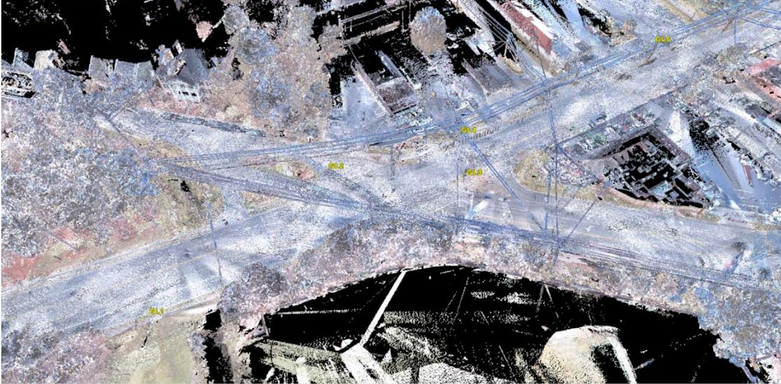
Figure 20 (a): Aerial View of Geo-Referenced Point-Cloud Model of City Intersection 2
