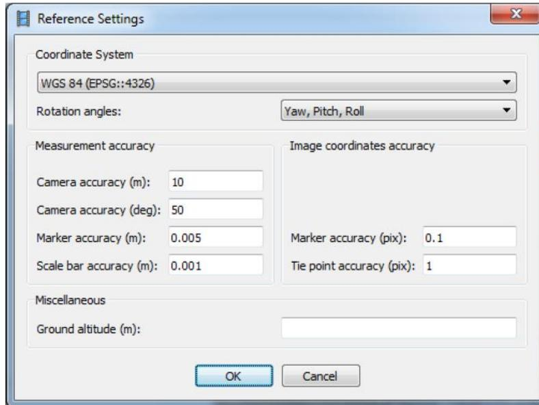
*Ground Altitude* should be specified in case of very oblique shooting and define the average ground altitude level above the ellipsoid in the selected coordinate system.
