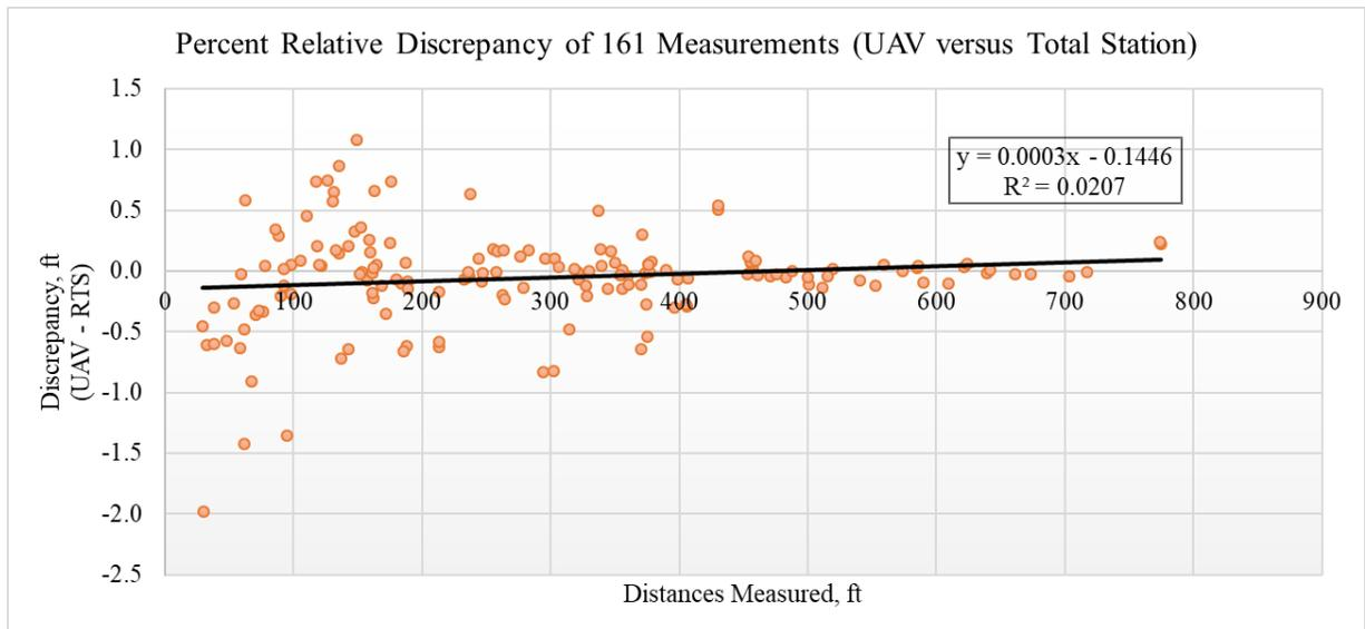
Figure H.7: Graph – Percent Relative Discrepancy with Recommended Camera Alignment Optimization from Agisoft PhotoScan (2017)
