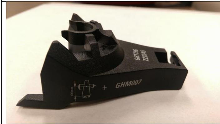
This clips to one on the tribrach knob poles and the end of the tape clip in to it.
