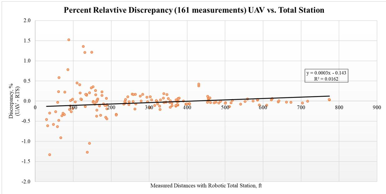
Figure H.5: Graph – Percent Relative Discrepancy of 161 Measurements (UAV versus Total Station)
