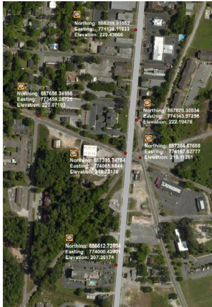
Figure 9: GPS Coordinates of Selected Control Points (Provided by the Georgia Southern Physical Plant)
