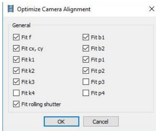
Figure G.7: Example of Optimize Camera Alignment Settings recommended by Agisoft PhotoScan (2017) for DJI Cameras
