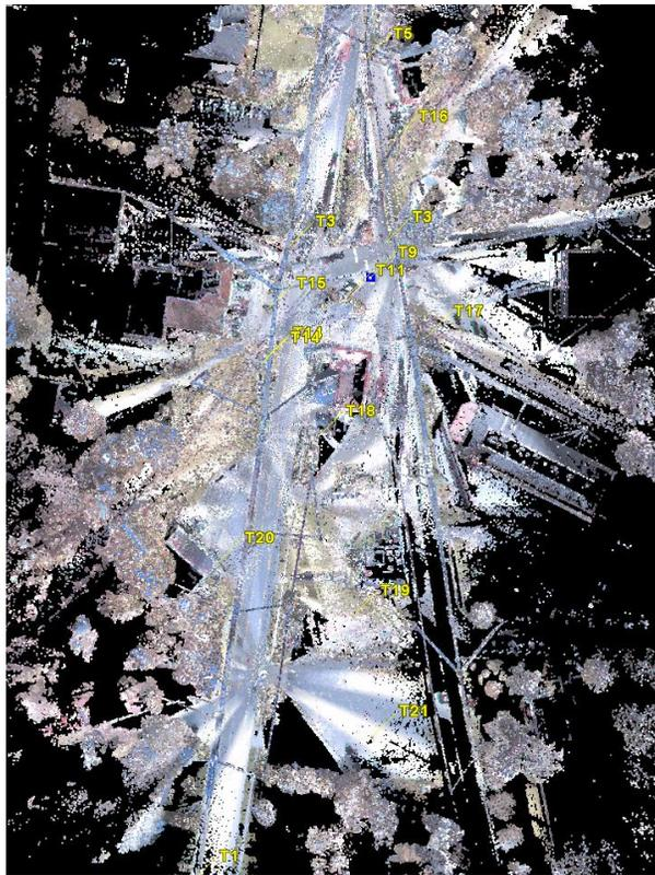
Figure 12 (a): Aerial View of City Street Intersection 1 Point Cloud Model
