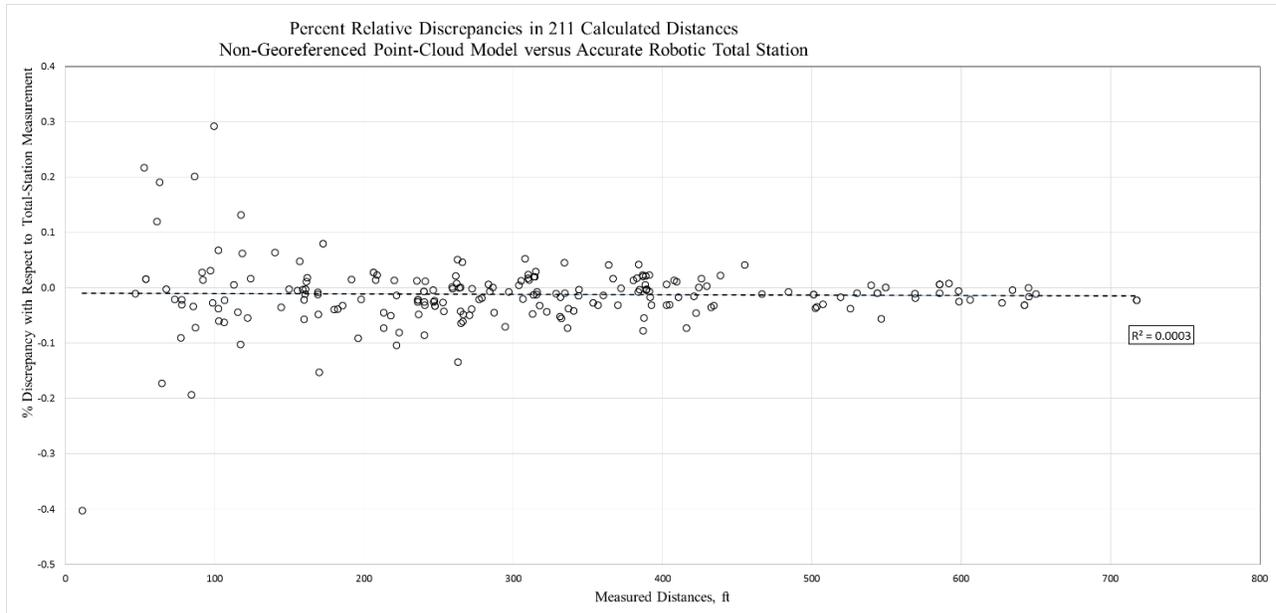
Figure H.1: Graph – Percent Relative Discrepancies in 211 Calculated Distances Non-Georeferenced Point-Cloud Model vs. Accurate-Robotic Total Station
