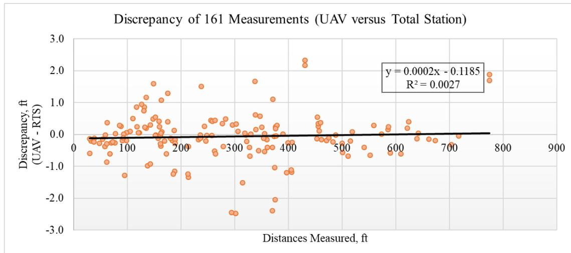
Figure G.10: Graph – Distance Discrepancy with Recommended Camera Alignment Optimization from Agisoft PhotoScan (2017)
