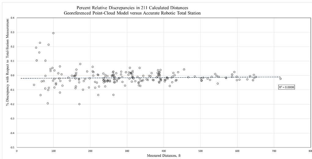
Figure 32: Graph – Percent Relative Discrepancies in 211 Calculated Distances Georeferenced Point-Cloud Model vs. Accurate-Robotic Total Station
