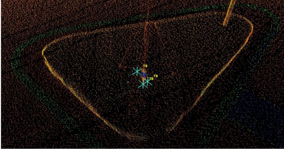
Figure 16: Multiple Targets of Control Point T9 in Visually Aligned Point-cloud Model
