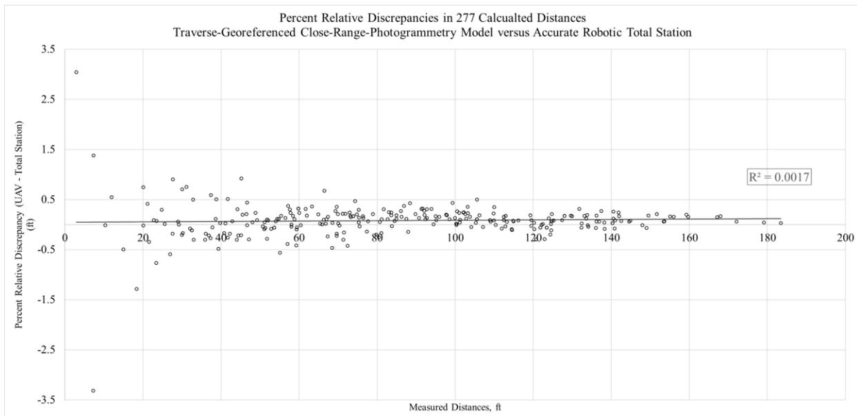
Figure H.8: Graph – Percent Relative Discrepancy in 277 Calculated Distances Traverse-Georeferenced Close-Range Photogrammetry Model versus Accurate Robotic Total Station (Building Structure with Parking Lot Infrastructure and Topography)
