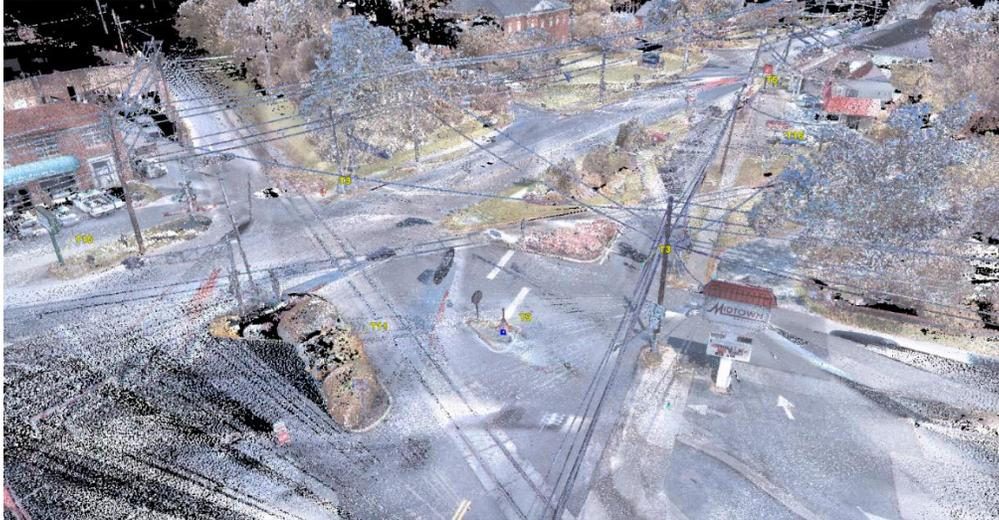
Figure 12 (b): Aerial View of City Street Intersection 1 Point Cloud Model
