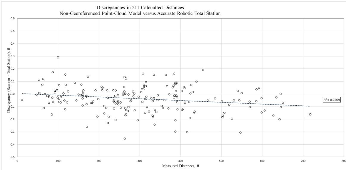
Figure 29: Graph – Discrepancies in 211 Calculated Distances Non-Georeferenced Point-Cloud Model versus Accurate Robotic Total Station
