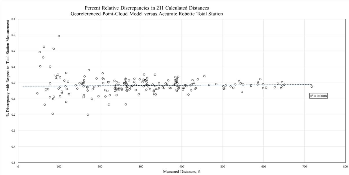
Figure H.2: Graph – Percent Relative Discrepancies in 211 Calculated Distances Georeferenced Point-Cloud Model vs. Accurate-Robotic Total Station
