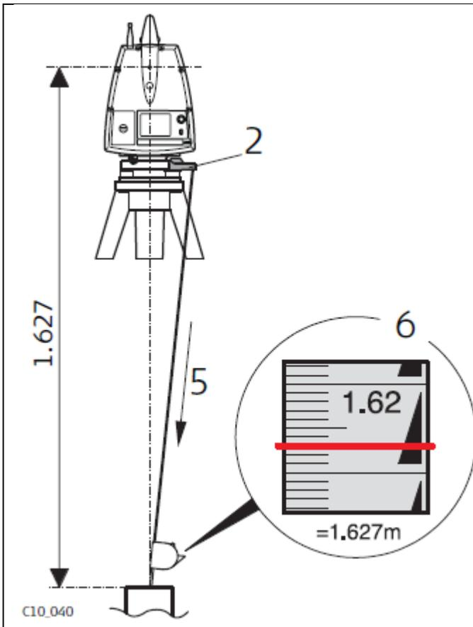
1. Place tripod centrally over the ground point, level instrument.
