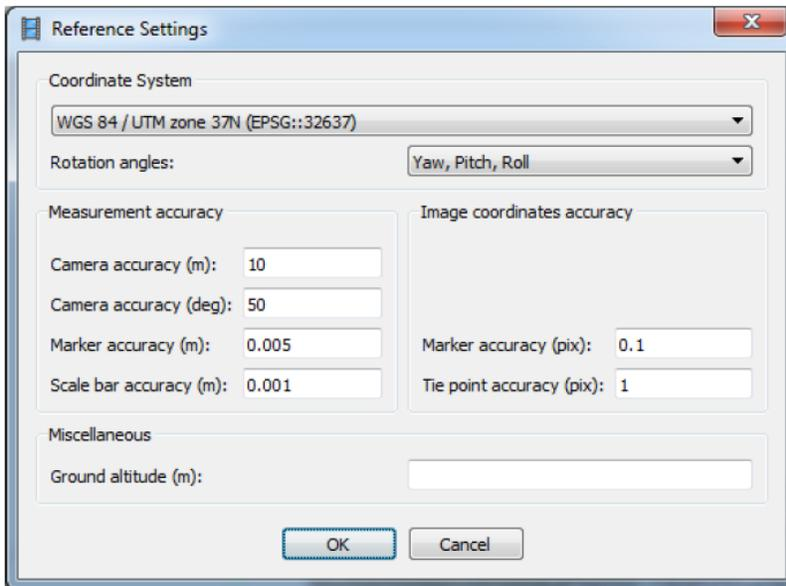
**Marker accuracy:** *0.005* (specify value according to the measurement accuracy).
