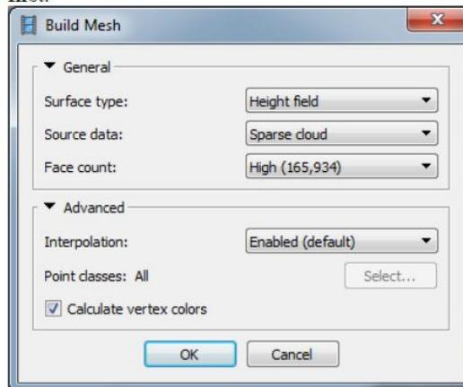
Select *Build Mesh* command from the *Workflow* menu and specify following parameters in the *Build Mesh* dialog:
