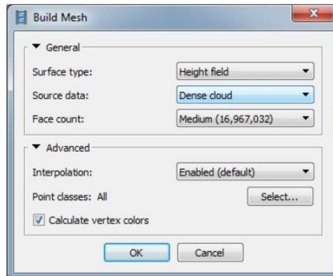
Set the following recommended values for the parameters in the *Build Mesh* dialog:
