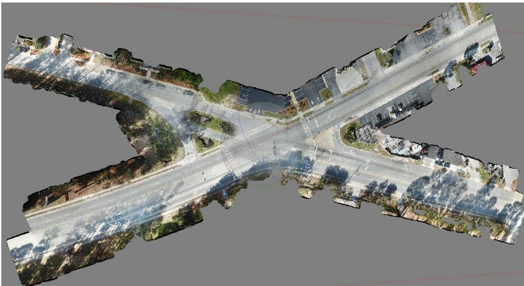
Figure 22 (a): Aerial View of 3D Dense-Cloud Photo-Based Model of City Intersection 2
