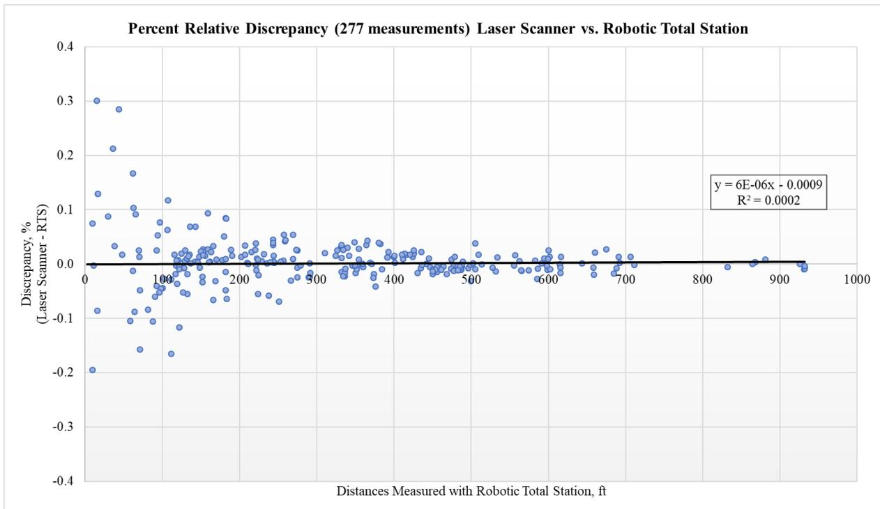
Figure H.4: Graph – Percent Relative Discrepancy of 277 Measurements (Laser Scanner versus Robotic Total Station)
