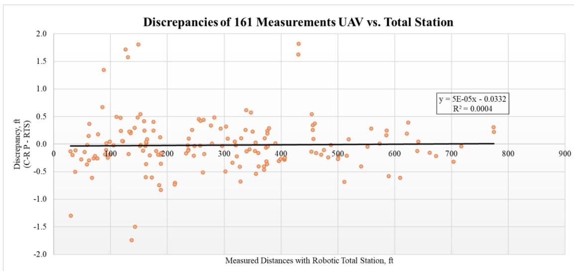
Figure G.3: Graph – Discrepancy of 161 Measurements (UAV versus Total Station)
