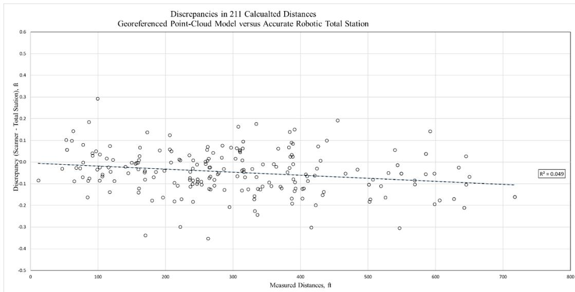
Figure 30: Graph – Discrepancies in 211 Calculated Distances Georeferenced Point-Cloud Model versus Accurate Robotic Total Station
