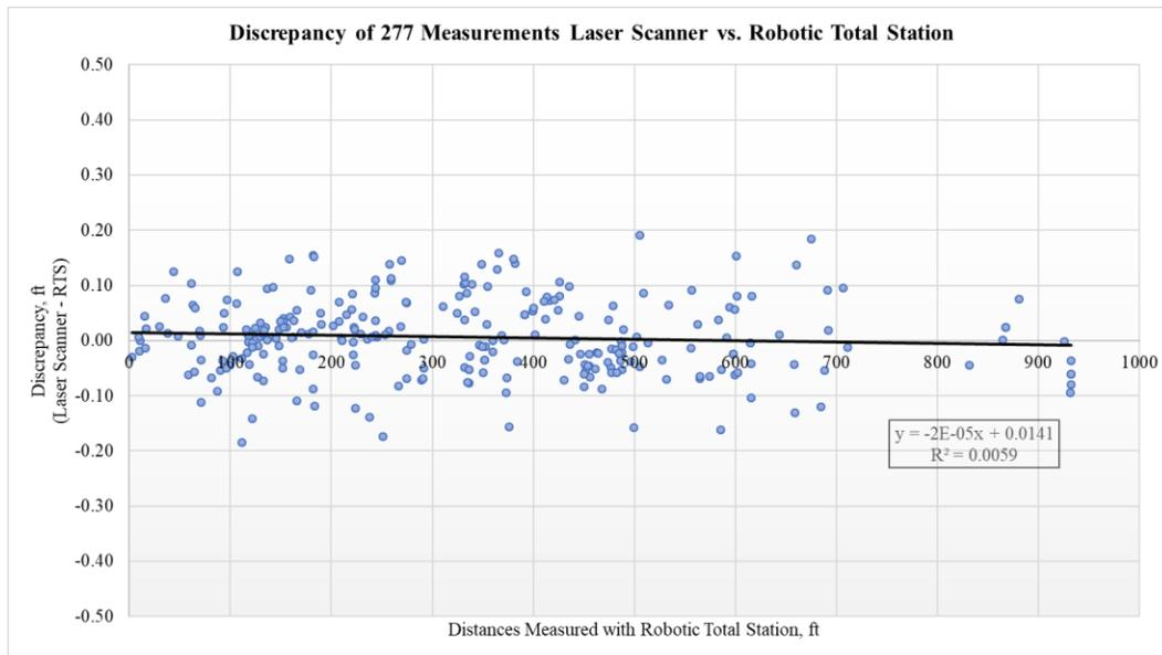
Figure 33: Graph – Discrepancy of 277 Measurements (Laser Scanner versus Robotic Total Station)
