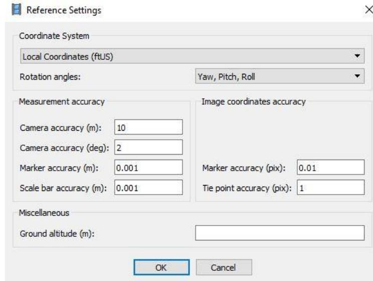
Figure 25: Default Accuracy Settings used for Photo-Based Model of City Intersection 2
