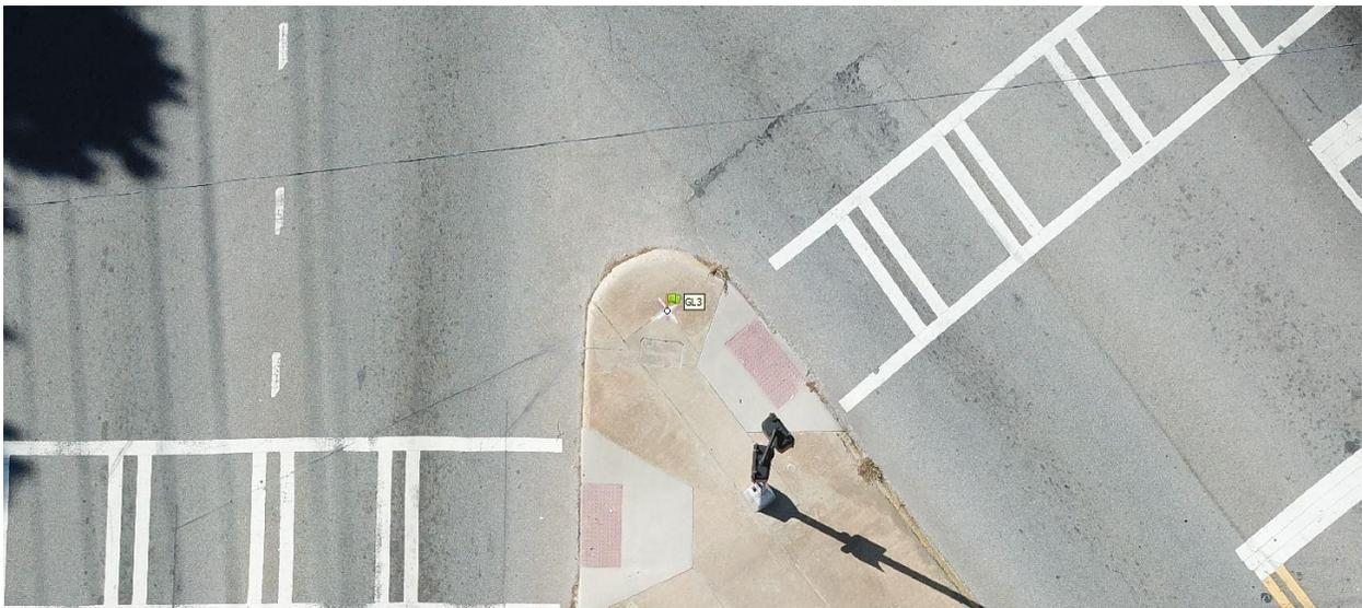
Figure 23: Marker Placement for Sample Point/Ground Control Point for Photo-Based Model of City Intersection 2
