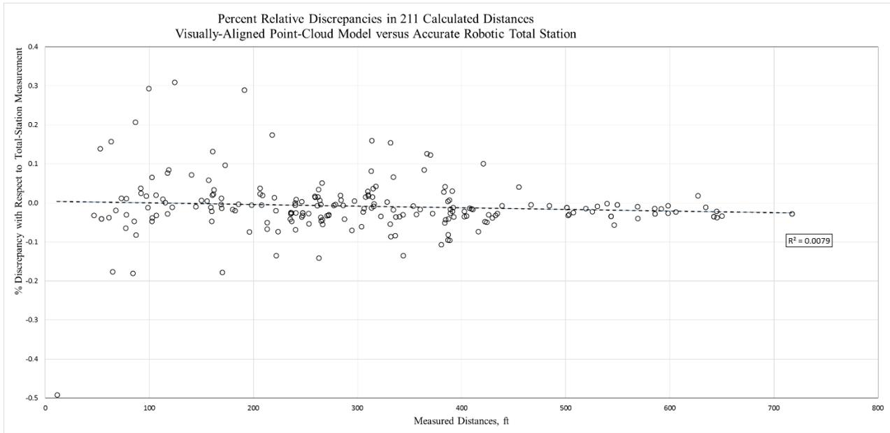
Figure H.3: Graph – Percent Relative Discrepancies in 211 Calculated Distances Visually-Aligned Point-Cloud Model vs. Accurate-Robotic Total Station
