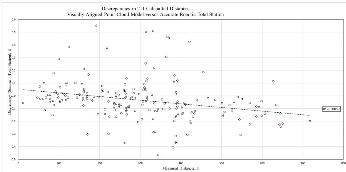
Figure 31: Graph - Discrepancies in 211 Calculated Distances Visually-Aligned Point-Cloud Model versus Accurate Robotic Total Station
