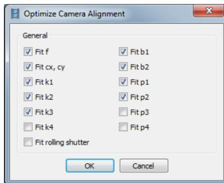
Select camera parameters you would like to optimize. Click *OK* button to start optimization process. (For DJI drone cameras it is usually suggested to optimize the rolling shutter).
