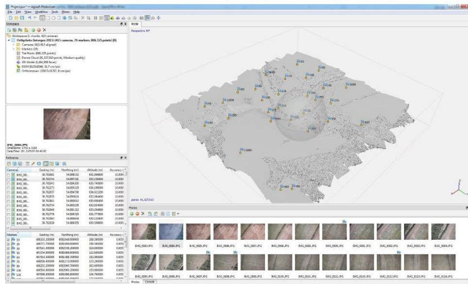
Points from the dense cloud can be removed with the help of selection tools and *Delete/Crop* instruments located on the Toolbar.
