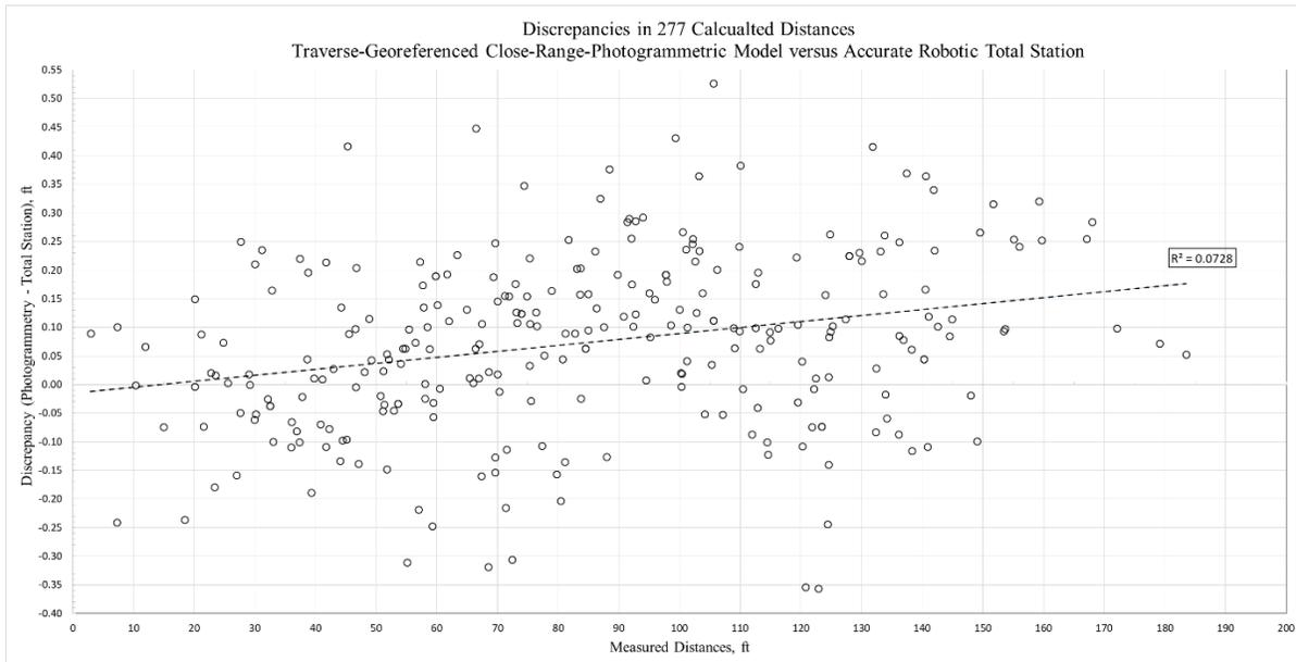
Figure 35: Graph – Discrepancies in 277 Calculated Distances Traverse-Georeferenced Close-Range Photogrammetric Model versus Accurate Robotic Total Station
