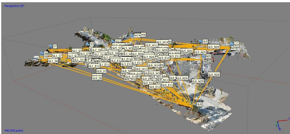
Figure 27: Distances Measured in PhotoScan for Photo-Based Model of City Intersection 2
