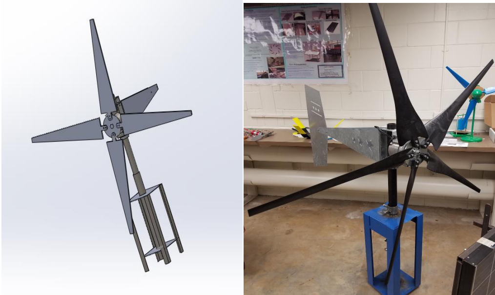
Figure 4A. CAD and Fabricated Model of New HAWT Blades Design Testing Unit.
