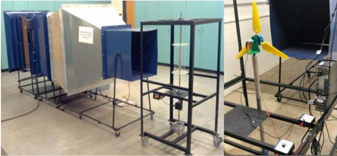
Figure 3.10. Wind Tunnel Configuration for HAWT and VAWT Testing
