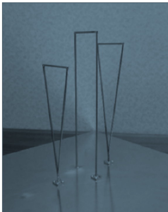
Figure 1-13. Yagi antenna with enhanced bandwidth (Arceo, 2011)
