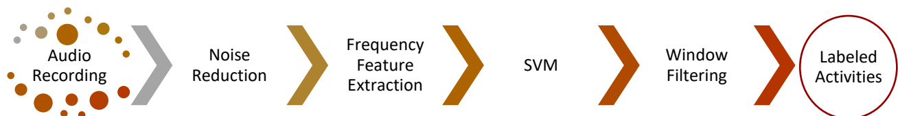
Figure 3.2: Machine learning model for audio signal processing.
