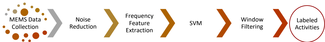
Figure 3.8: Machine learning model for MEMS accelerometer data processing.
