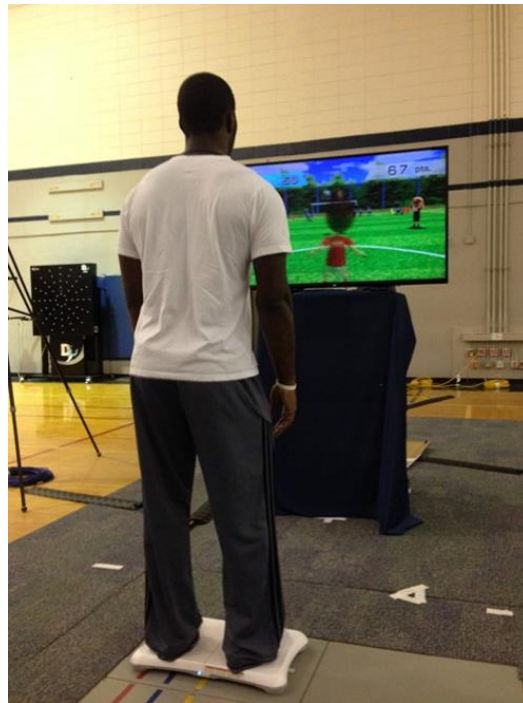
Figure 5: Subject using the Wii Balance Board (WBB) and Wii Fit Soccer Heading Game, in playing position
