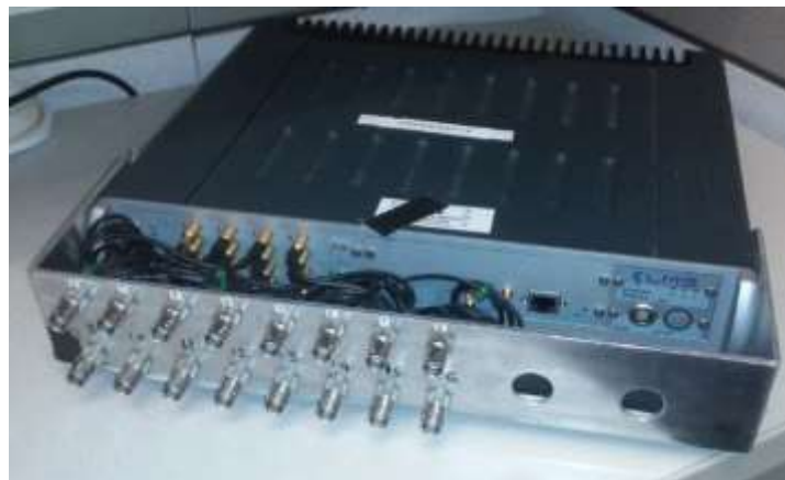
Figure 3.9. LMS SCADAS mobile DAQ system with BNC connectors attached
