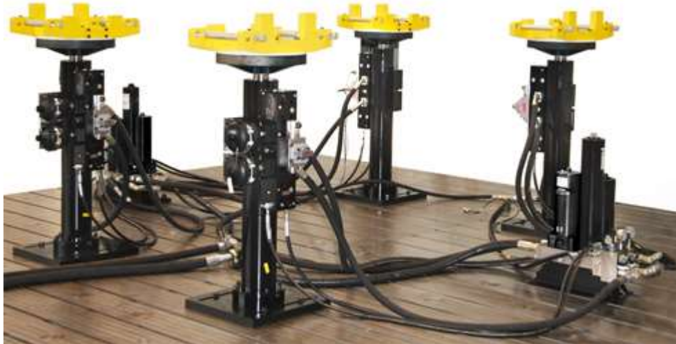
Figure 3.13. A hydraulic 4 poster test rig
