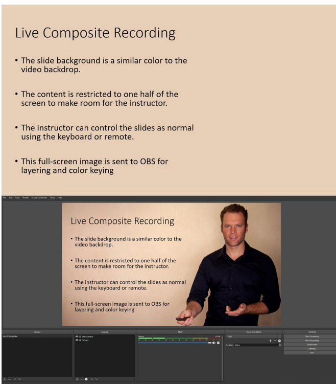
Figure 2. Screen capture of dual-monitor setup in OBS Studio. The full-screen slide content (top) and camera video signal are combined in OBS Studio (bottom).
