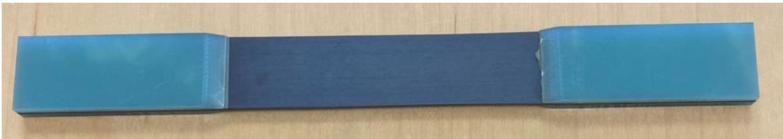
Figure 1. Unidirectional Carbon Fiber Reinforced Polymer
