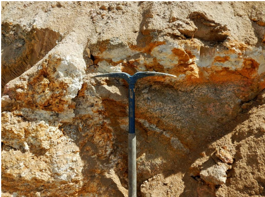
Fig. 15. Saprolite from Hanson Quarry with kaolin-rich zone above it. Note preserved granite texture in saprolite.
