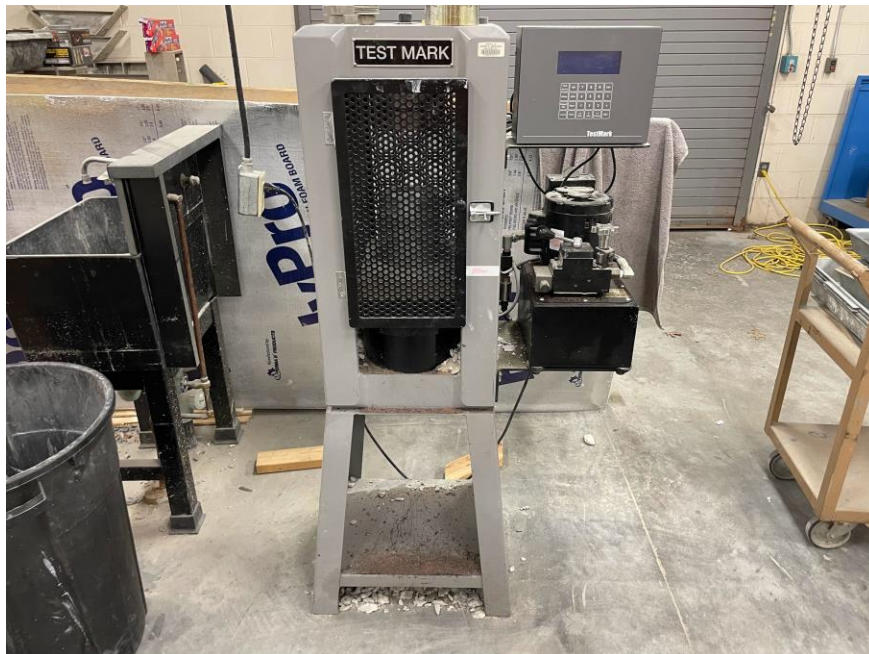
Figure 3. Concrete Compression Test Machine
