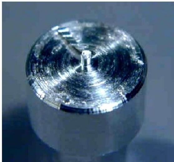
Figure C5: Surface profile of the disk after parting operation
