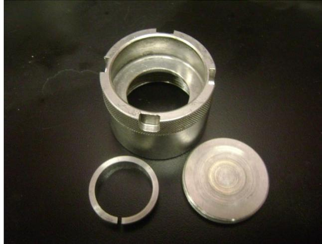
Figure 34: Components of the disk holding assembly
