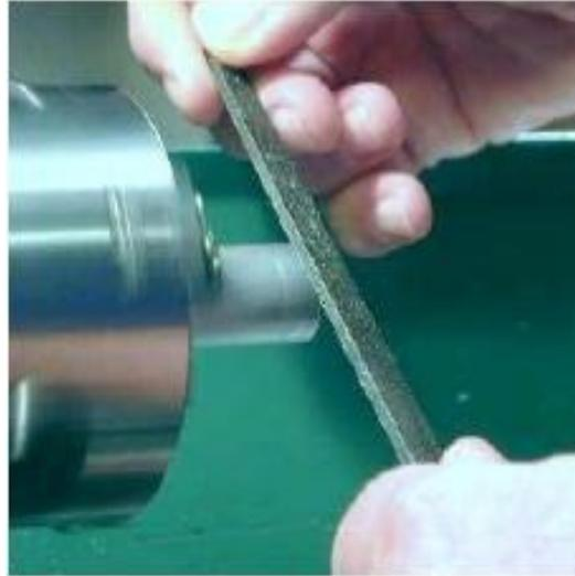
*Figure C6: Chamfering the work- piece edges with file.*
