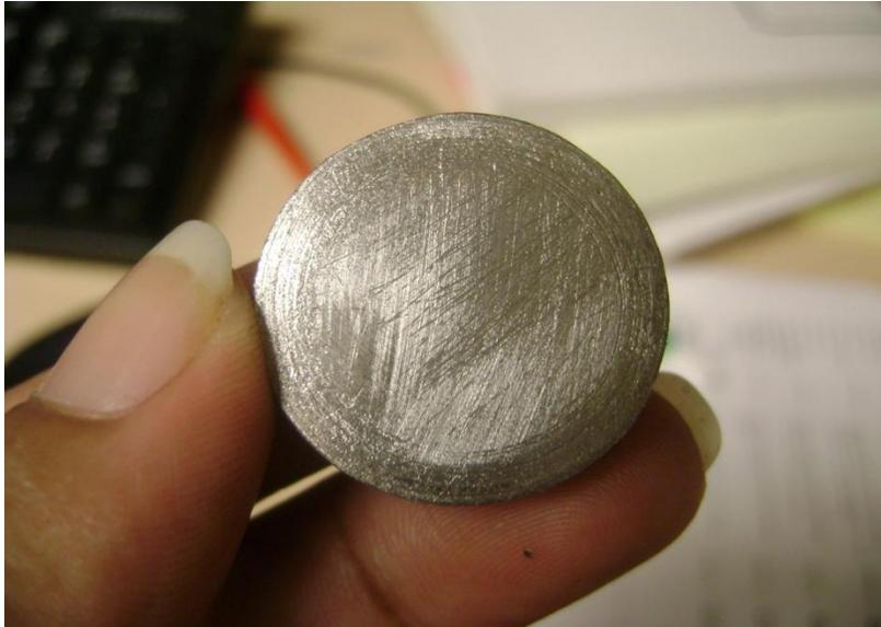
*Figure C7: Surface of the disk after polishing with file*
