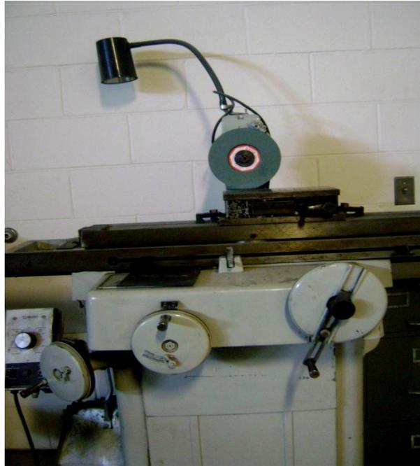
*Figure C8:* Surface grinder used for surface finish.
