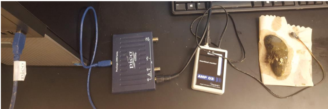
Figure 3. Set-up for heart rate measurements; mussel, IR sensor, amplifier, Picoscope, and computer (right to left).
