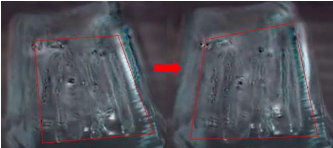
Figure 7: Magnified Mode Shape for Healthy Cube
