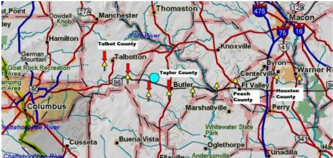
Figure 5. A detailed map of the 230kV transmission line (denoted by arrows pointing up) beginning in Warner Robins, GA and ending in Talbotton, GA. In the spring of 2004, the line extending west from Butler, GA was replaced with non-tubular cross-armed towers (denoted by arrows pointing down).
