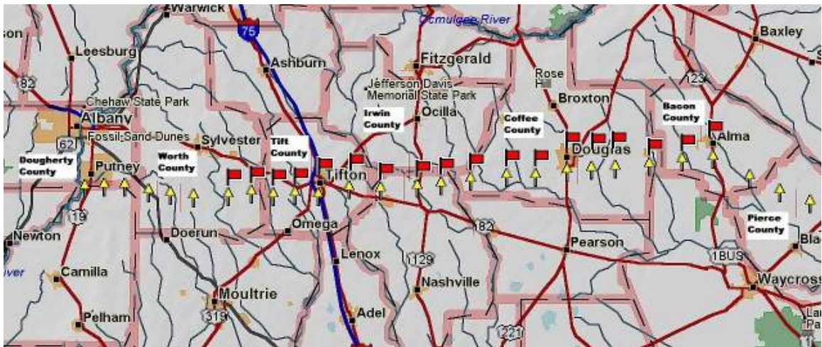
Figure 2. A detailed map of the 230kV transmission line running from Offerman, GA, to Putney, GA (denoted by arrows). The eastern side of the single line begins in Offerman and ends in Alma when another power line (denoted by flags) begins to run parallel to the study line until it reaches Tifton, where it becomes single again until the end in Putney.
