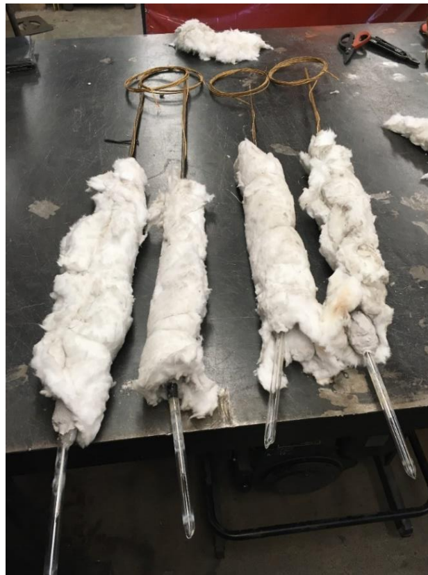
Figure 5: Quartz Mold Assemblies for Fast-Quench Grey Iron Samples
