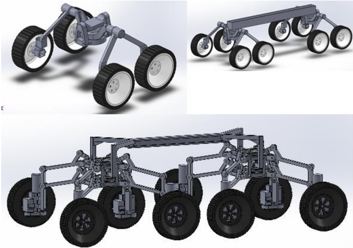
Figure 3: Early CAD model of a wheel pod with the three degree of freedom joint to allow roll, steering, and pitching of the robot, and the connection between the two pods to form the chassis. On the bottom is the updated model.
