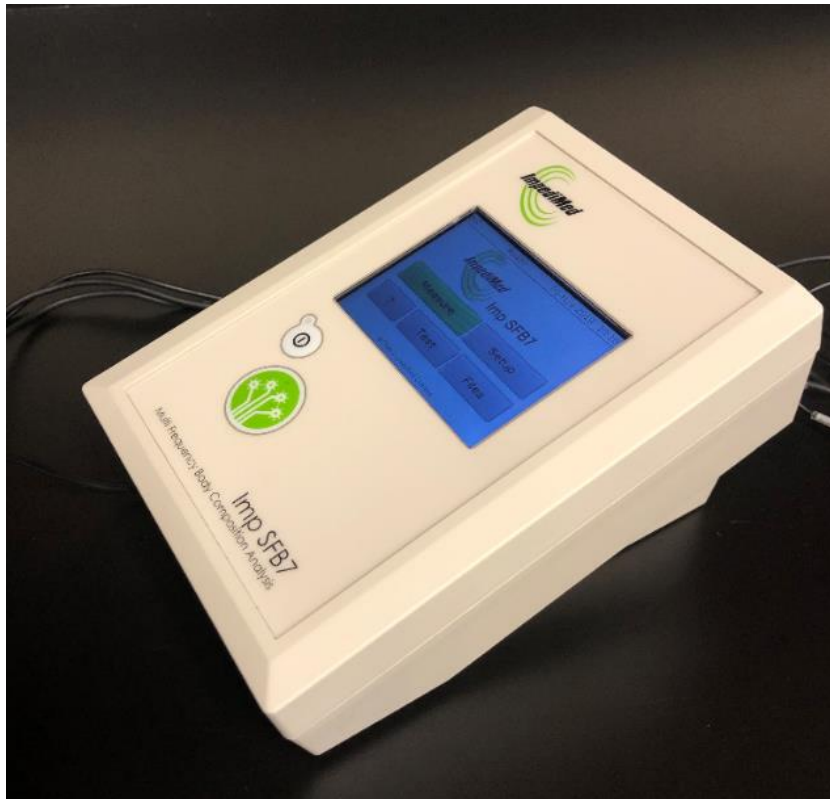
Figure 4: The SFB7 device used to collect the resistance readings can be seen in the figure.
