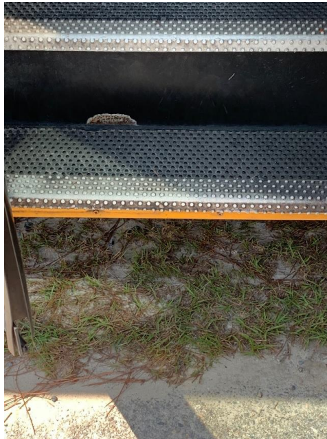
Figure 3. School bus step height that makes it difficult for children to climb up independently
