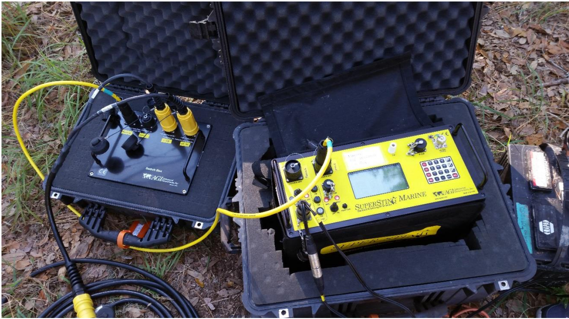
Figure 11: Image of the Supersting Marine control systems. Personal image.
