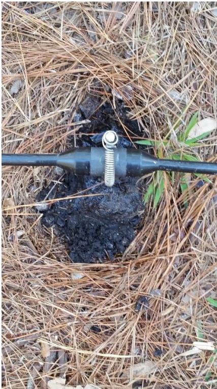
Figure 12: Electrical resistivity node that has been staked to the ground and surrounded by saltwater on St. Catherines Island. Personal image.
