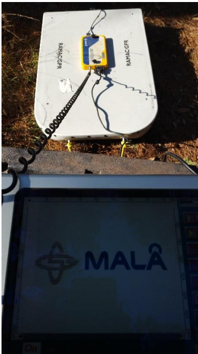
Figure 4: GPR set-up using 100 MHz antenna being dragged behind a John Deer Gator. Personal Image.
