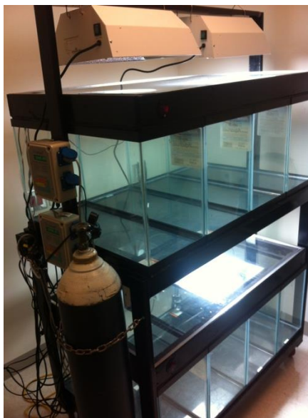
Figure 1. The AtmoSim2100; an elevated CO 2 atmospheric simulator
