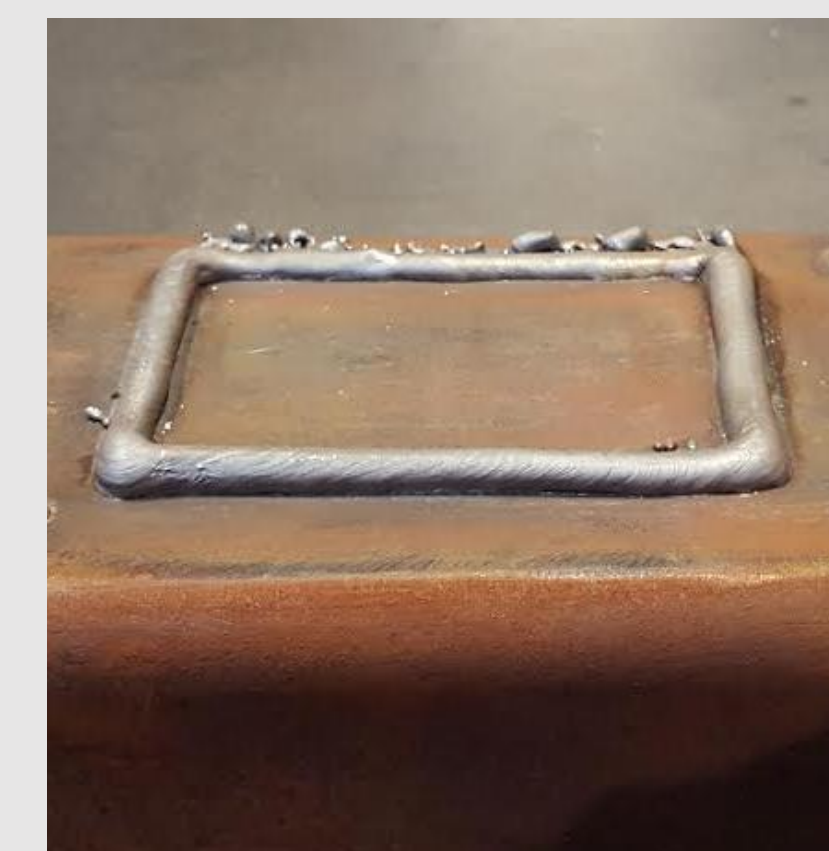
Four layer(.070") square created by WAAM process
