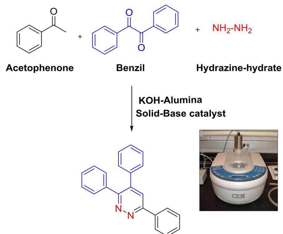
Figure 1. Multicomponent organic reaction for the microwave-assisted solvent-free synthesis of 3,4,6-trisubstituted pyridazine derivatives. The CEM discover microwave reactor is shown in the inset.
