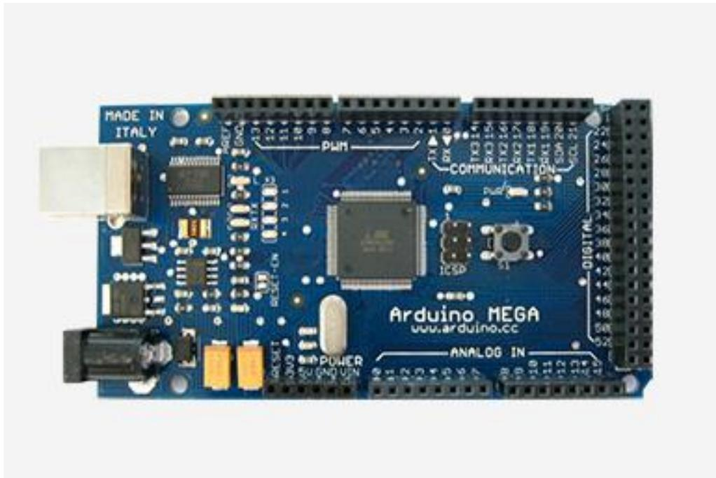
Figure 11: Microcontroller Used to Interface the Laptop and Arm [12]
