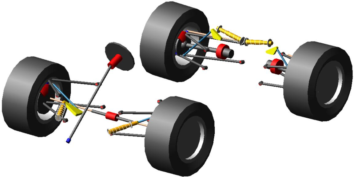
Figure 4 – Full Vehicle Assembly modeled using Adams/Car software.
