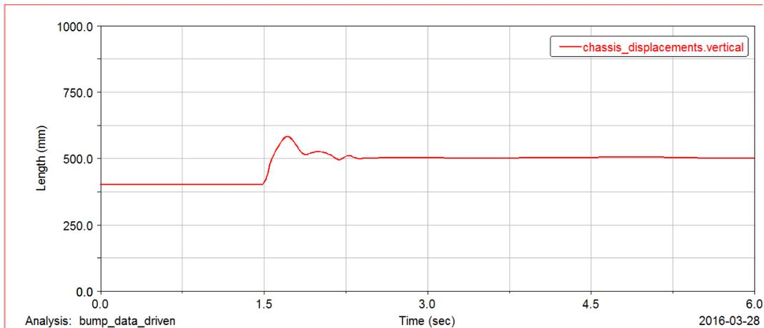
Figure 18 – Vertical Chassis Displacements (10 cm Road Bump)
