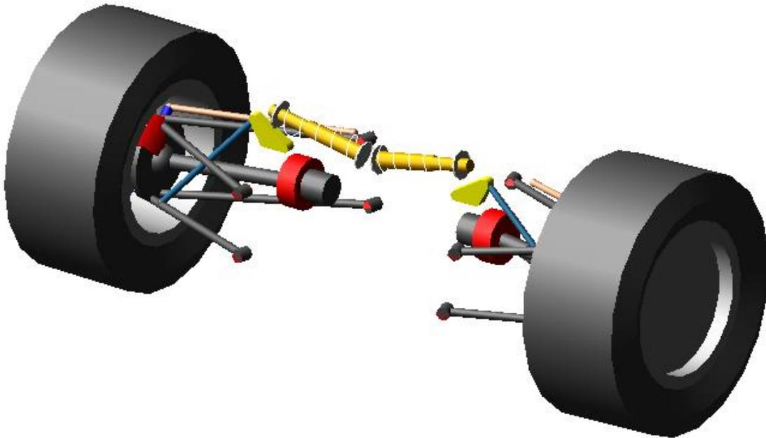
Figure 3 – Rear Suspension Assembly, complete with powertrain and brakes.
