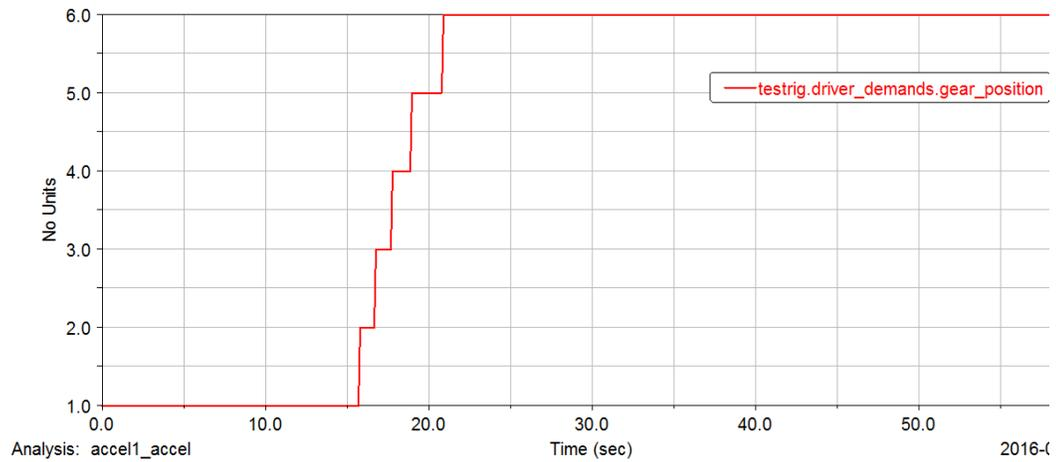
Figure 16 – Gear Position v. Time (Straight Line Acceleration)
