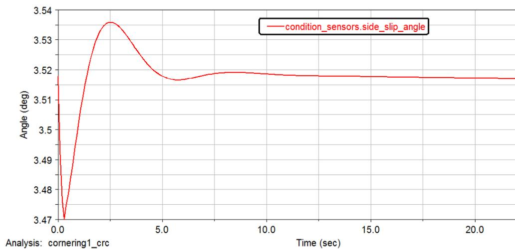
Figure 6 – Side Slip Angle v. Time (Constant Radius Cornering, 20m radius, 20km/hr)
