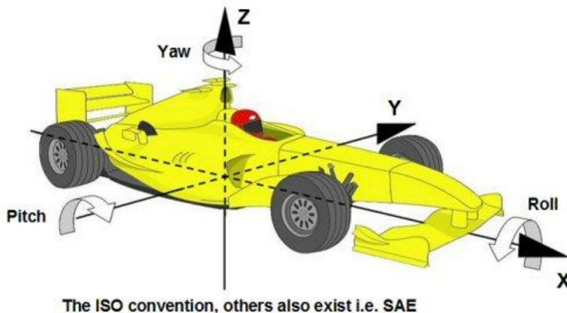
Figure 1- Roll, Yaw, and Pitch Diagram
