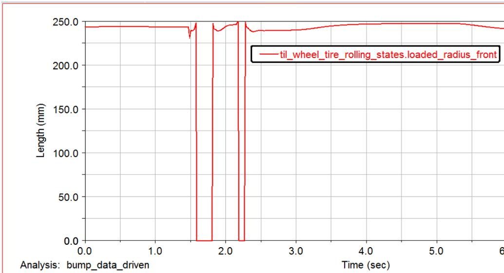
Figure 22 – Front Tire Loaded Radius (Straight Line Acceleration)
