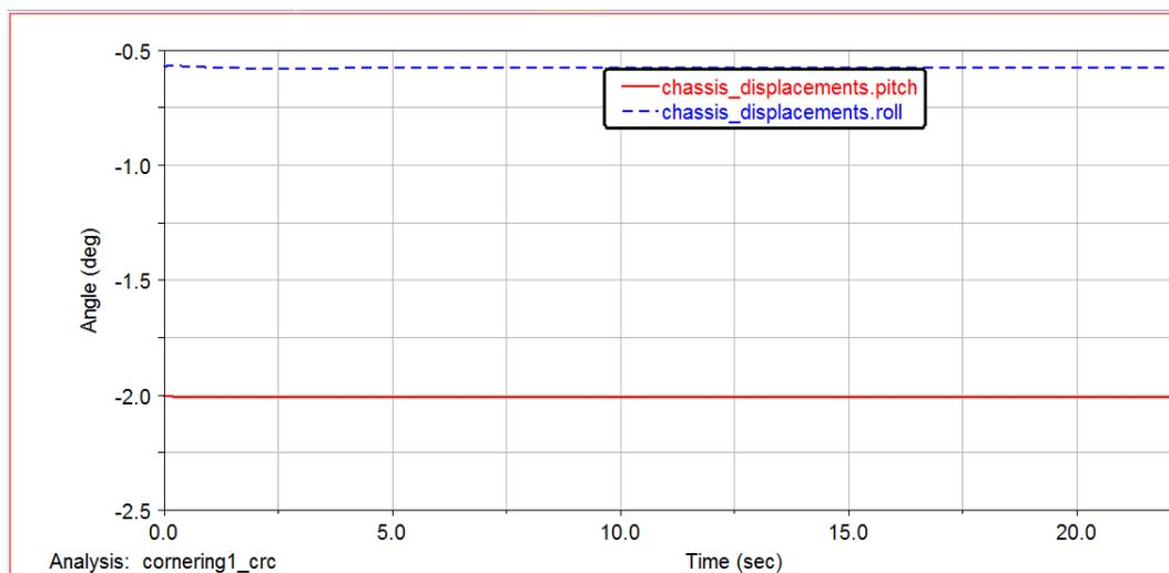
Figure 5 – Roll and Pitch Angle v. Time (Constant Radius Cornering, 20m radius, 20km/hr)
