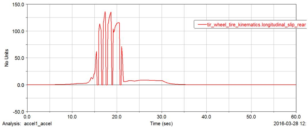
Figure 12 – Rear Wheel Slippage v. Time (Straight Line Acceleration)
