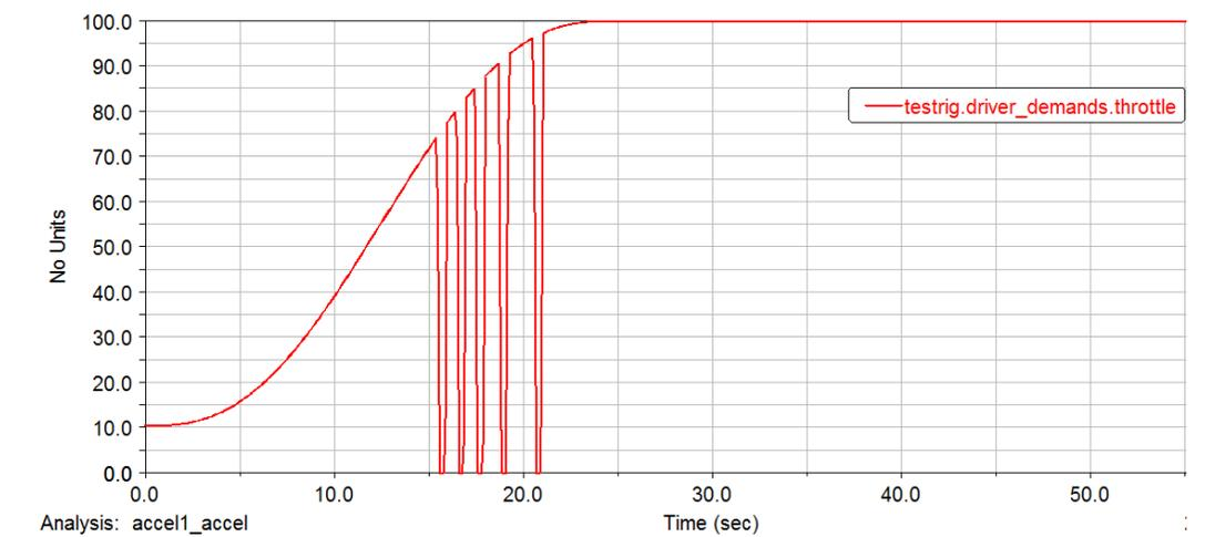
Figure 15 – Throttle Demand v. Time (Straight Line Acceleration)
