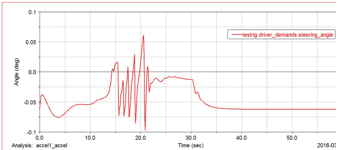
Figure 17 – Steering Wheel Angle v. Time (Straight Line Acceleration)
