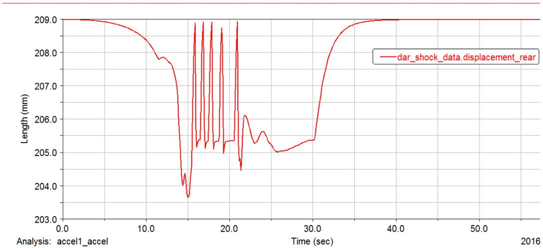
Figure 13 – Rear Shock Displacement v. Time (Straight Line Acceleration)
