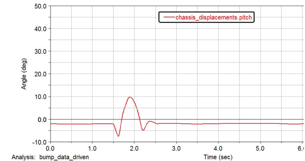
Figure 19 – Chassis Pitch Angle (10 cm Road Bump)
