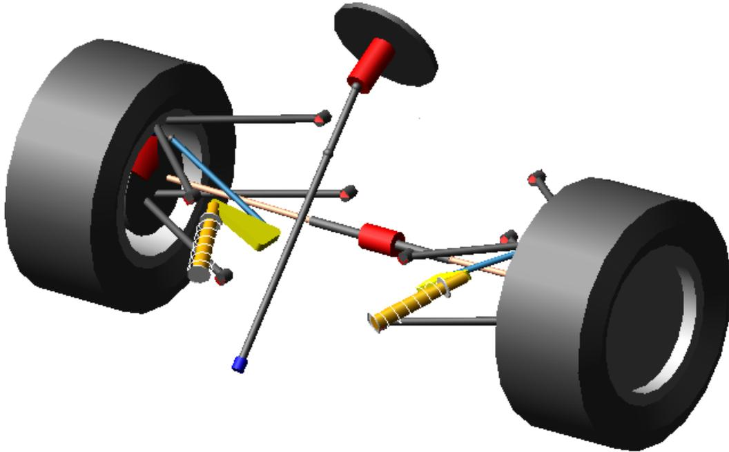
Figure 2 – Front Suspension Assembly, complete with steering subassembly and brakes
