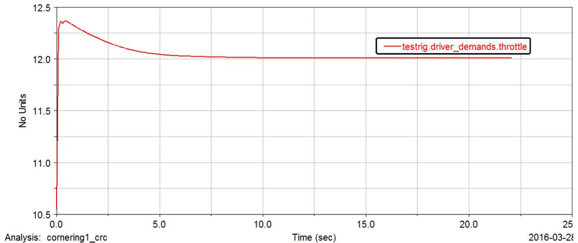
Figure 8 – Throttle Demand v. Time (Constant Radius Cornering, 20m radius, 20km/hr)
