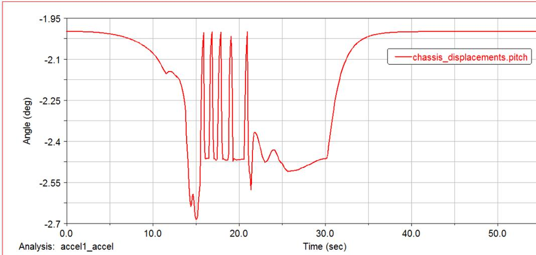
Figure 10 – Pitch angle v. Time (Straight Line Acceleration)
