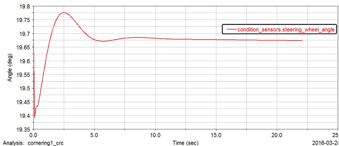
Figure 7 – Steering Wheel Angle v. Time (Constant Radius Cornering, 20m radius, 20km/hr)
