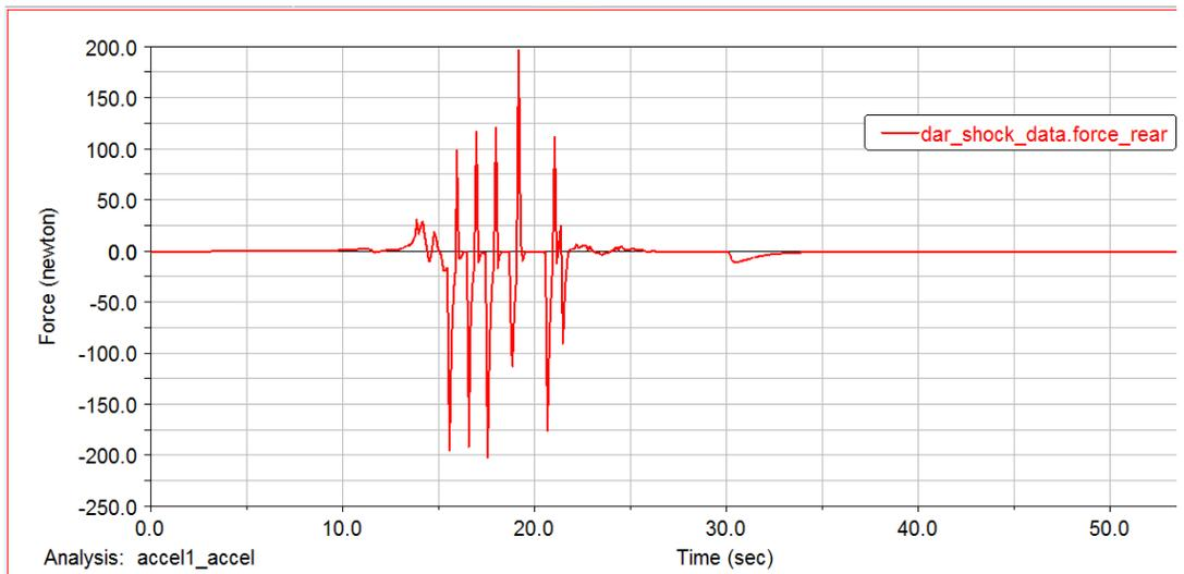
Figure 14 – Rear Shock Force v. Time (Straight Line Acceleration)
