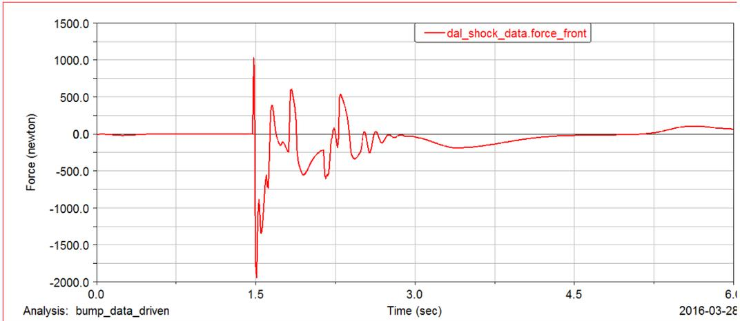
Figure 20 – Front Shock Force (10 cm Road Bump)
