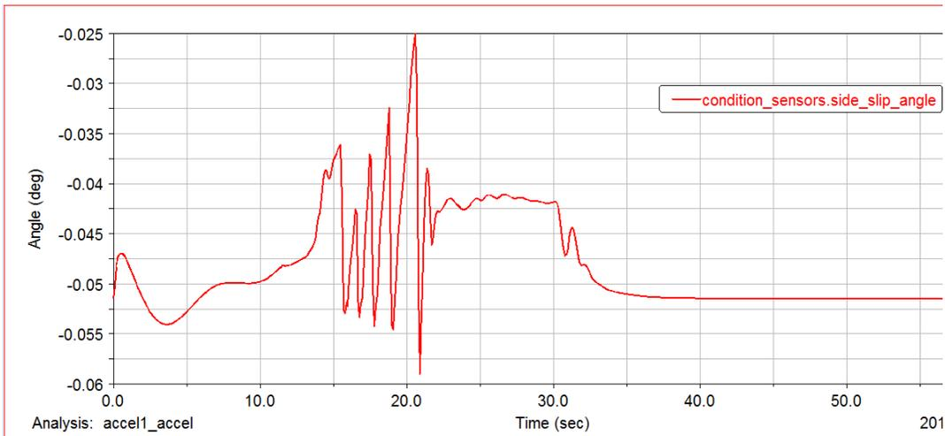
Figure 11 – Side Slip Angle v. Time (Straight Line Acceleration)
