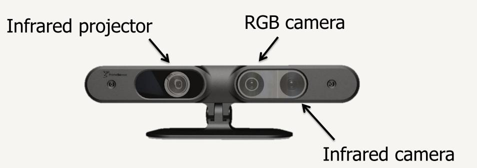
• A depth camera holds a large advantage over a color camera in many robotic applications. Instead of identifying objects based on color, objects are identified by pixel locations in space. In the images to the upper right, white pixels represent the closer objects to the camera while the black represents those that are farthest away. The projector emits an irregular pattern of infrared dots of varying intensities. The infrared camera recognizes the pattern and constructs a depth image.
