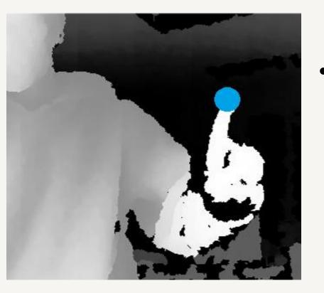
• To the left, is a screen capture of the program tracking the nearest pixel in the infrared image. A blue circle is drawn over the identified pixel.
