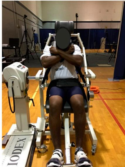
**Figure 2.** Core strength test setup on a dynamometer.
