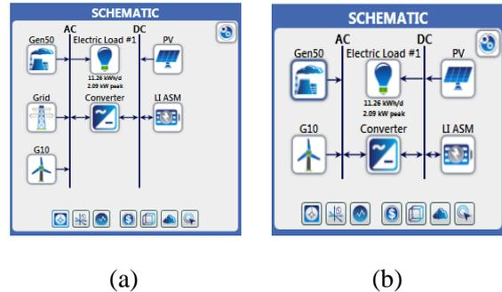
Fig. 2 Structure plan in HOMER (a) on-grid (b) off-grid
