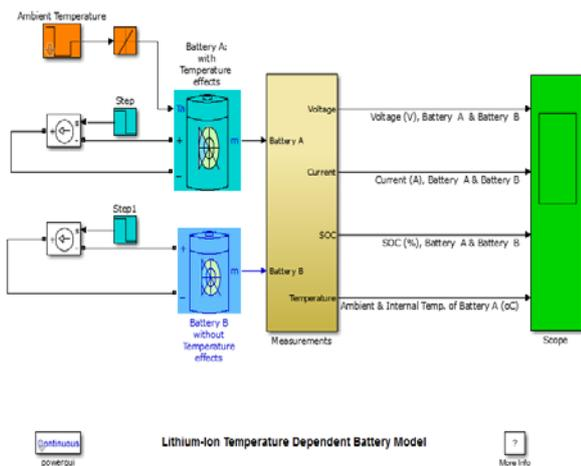
Fig. 3 Temperature dependent lithium-ion battery model
