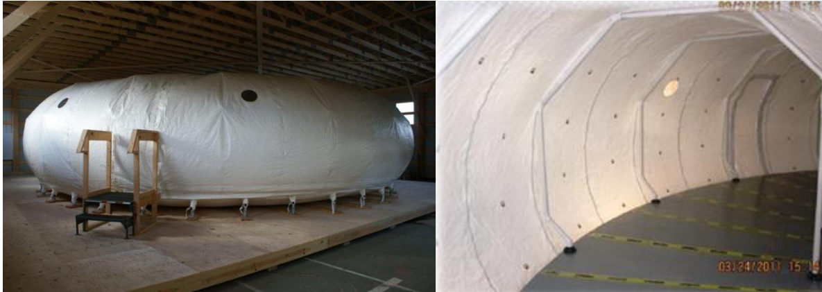
Figure 9. Exterior view (left) and inside view (right) of Inflatable lunar habitat (42 ft diameter 10 ft high concentric torus) designed and built by NASA JSC and instrumented with wireless sensors by University of Maine’s WiSe-Net Lab team.
