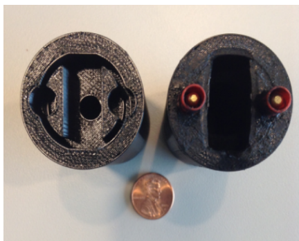
a) Printed Fuel Grain with Electrodes
