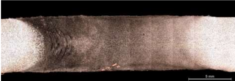
Figure 13. Optical microscopy image of an etched sample of a transverse SR-FSW made in 0.63 cm thick plates. Cu was plated on the AS root surface and is shown to have minimal entrainment into the weld nugget region.
