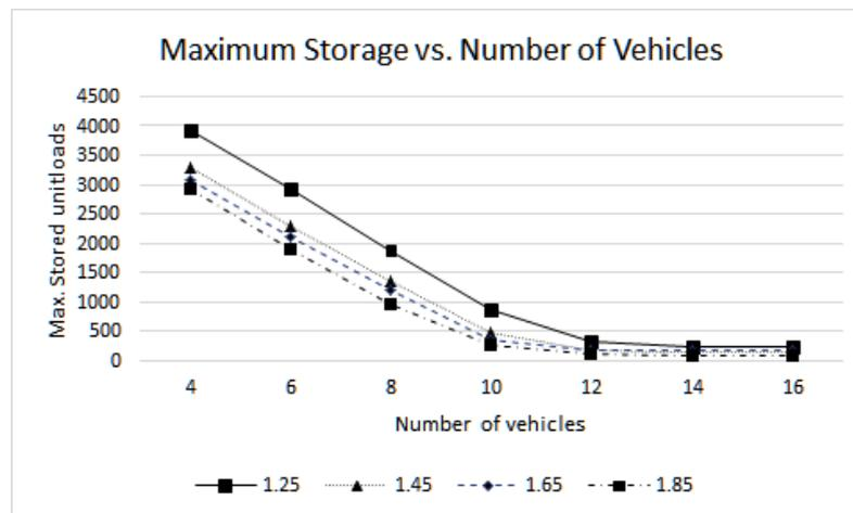
Figure 6: Maximum units stored, limited outbound capacity
