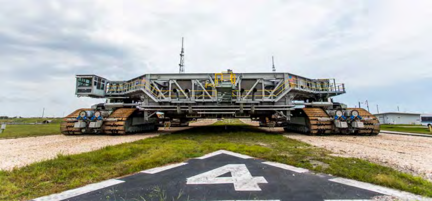
One of two “crawlers” at NASA, which carry the launch vehicle to the launch pad.
