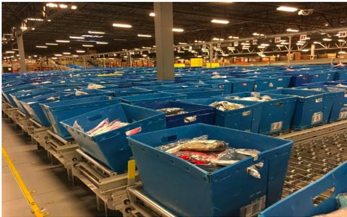
Fig. 3. Wave Bank. Totes are waiting at the wave bank ready to be released to the put walls for sortation
