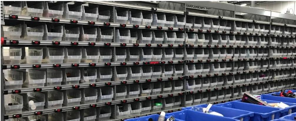
Fig. 2. A put wall. Each bin is dedicated to an order. Totes arrive carrying mixed SKUs. When an operator scans an item, the light under the bin where the item needs to be put lights up.
