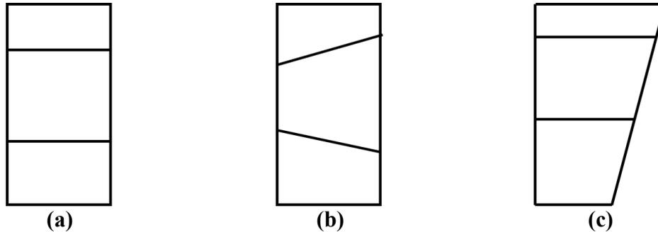
**Figure 4: Layout of a Single Bay (a) Before Aisles are Rotated; (b) With Horizontal Aisles Rotated; (c) With a Vertical Aisle Rotated.**
