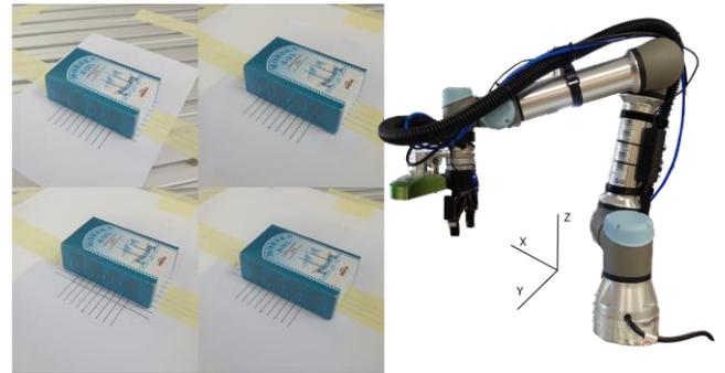
Fig. 2. The location of four points  $SP_1 (0, 0, 0)$ ,  $SP_2 (10, 0, 0)$ ,  $SP_3 (0, 10, 0)$ , and  $SP_4 (0, 0, -10)$  of the packed salt object and the coordinate system of the robot used in the experiments.
