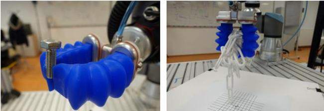
Fig. 13. Grasping of (a) bolt and (b) chain with soft robotic gripper.
