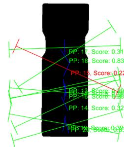
Fig. 16. Grasping score of the two-fingered robotic gripper for the door hinge object on selected object height  $h = 17.5$  mm.
