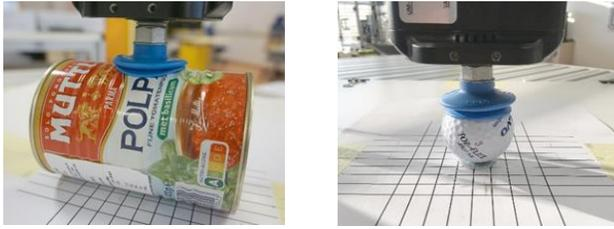
Fig. 8. Grasping of (a) tomato can and (b) golf ball with vacuum gripper.
