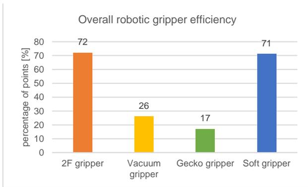
Fig. 4. Overall robotic gripper efficiency for selected objects.
