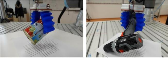
Fig. 12. Grasping of (a) can of tomatoes and (b) drill with soft robotic gripper.
