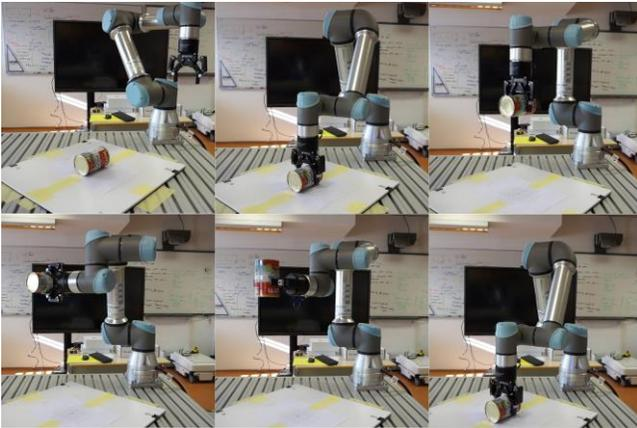
Fig. 3. The sequence of modified YCB Gripper Assessment protocol.
