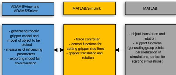
Fig. 14. Schematic of ADAMS/MATLAB co-simulation model.
