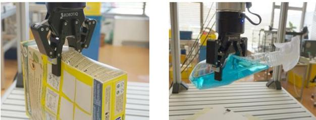
Fig. 6. Grasping of cereals box (a) and glass cleaner (b) with the two-fingered gripper.
