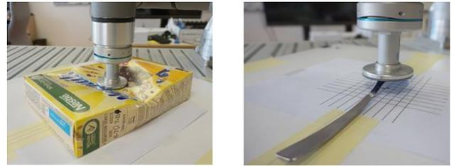
Fig. 10. Grasping of the (a) cereals box, and (b) spoon with the gecko robotic gripper.
