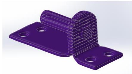
Fig. 15. Sliced door hinge model by layers in SolidWorks.
