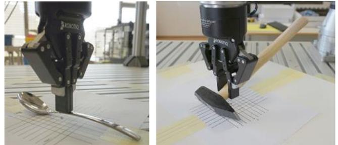
Fig. 7. Grasping of (a) spoon and (b) hammer with the two-fingered robotic gripper.
