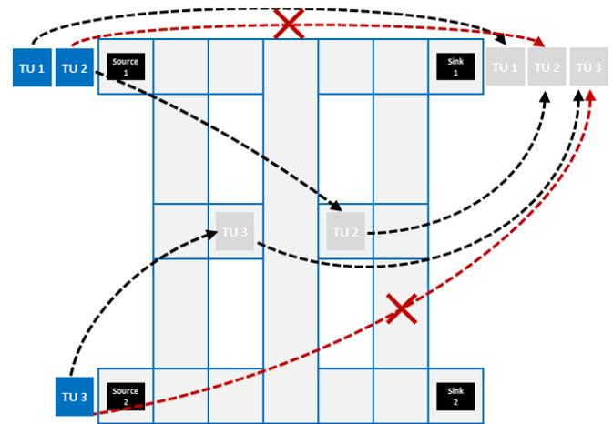
Fig. 4. Substitution of a workflow from a source to sink with two sub-workflows from a source via an intermediate to a sink aMFM.
