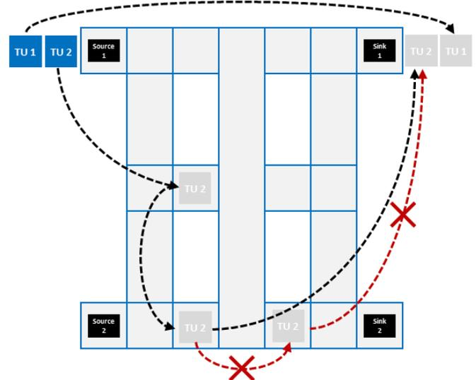
Fig. 5. Cancellation of a buffer aMFMs chain in order to arrive at a destination aMFM earlier than originally planned.
