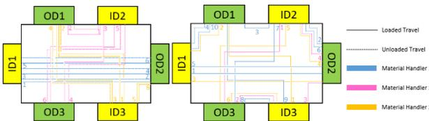
Fig. 1. Sample dedicated (left) and monomaniacal (right) unloading process
