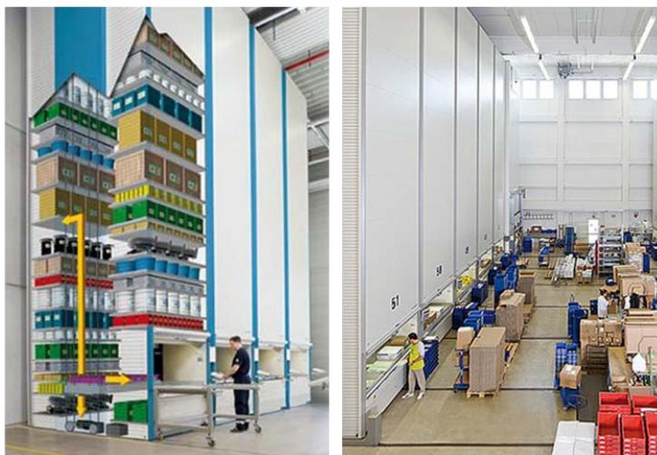
Figure 1. Vertical lift modules
