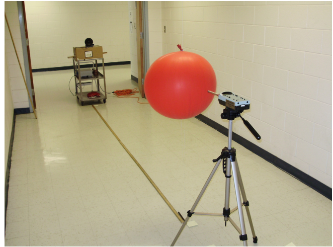
FIG. 5. (Color online) Experimental setup showing Brüel & Kjær Type 2230 Precision Integrating Sound Level Meter in “close” position.
