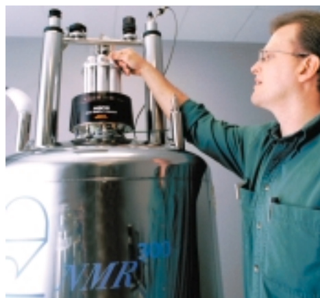
Richard Wallace places a sample into the new nuclear magnetic resonance spectrometer.
